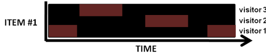
Figure 10. Stack of three visitor stripes in the first item row where the red color denotes their residing time intervals near item 1.
